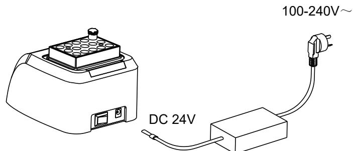
1.3.3 Power on the main switch. The incubator is ready to operate when the display becomes visible.
