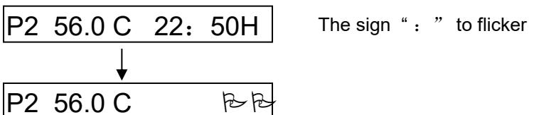
When the time count down to "00:00", it will display "~~~~", and the buzzer alarm "du. du." 2 voices. If the program P8 is over , the buzzer will alarm "du.du. ...du." 8 voices, and so on.
